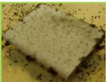
The uncoated panel is covered with mold growth.
