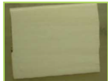
The Energy Protect™ coated panel has zero mold growth.
