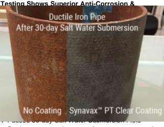
Study, zero corrosion on surface, even at scored areas, no loss of adhesion.
