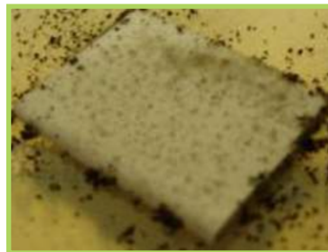
Uncoated panel: Covered with mold growth.
