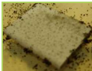
Uncoated panel: Covered with mold growth.
